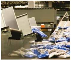
**BULK FLOW** Robust bed frame, high side guides and pre-engineered dump points enable reliable, jam-free conveyance of a wide variety of bulk material.
