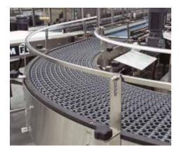
CASEMAT<sup>™</sup> AND ACCUMAT<sup>®</sup> Modular plastic belts provide rollerless accumulation and transportation through curves, straights, inclines and declines.
